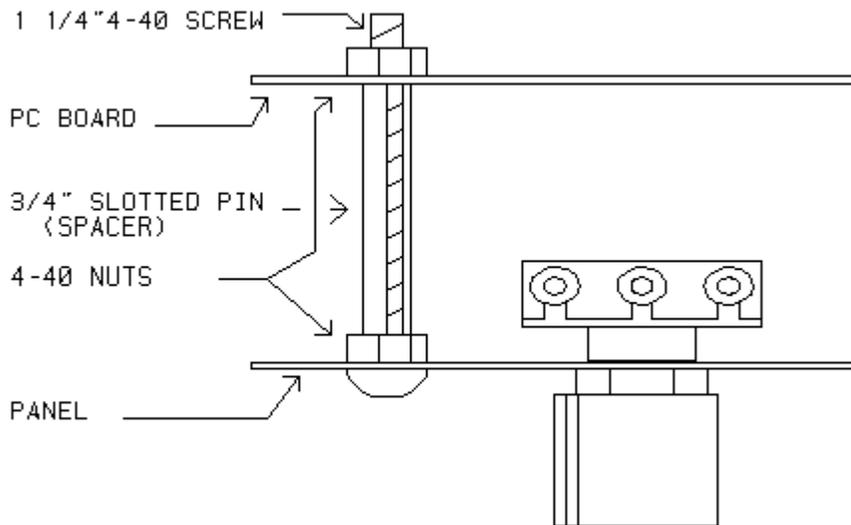
Follow the wiring diagrams in order; first the top row of controls, then the middle and bottom. Be sure to leave enough slack in the wires to easily place the board back on the spacers over the controls. Secure the board in place with 4-40 nuts.
